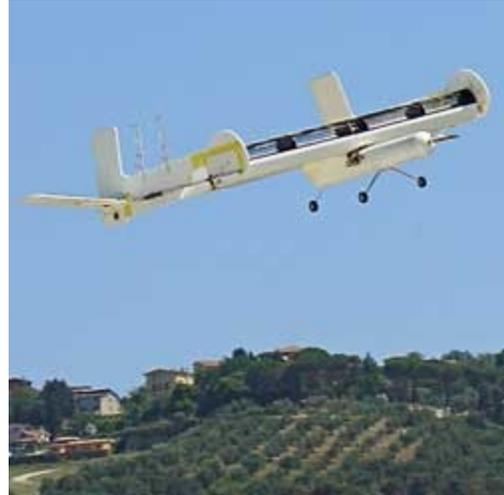
A scale-model remote-control FanWing has been flying in Italy. © FanWing Ltd. 2011
