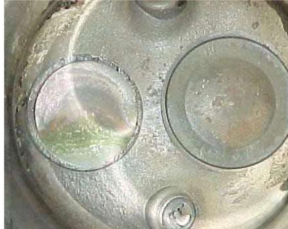
This is a healthy cylinder head. The exhaust valve has a “symmetrical red” pattern that is good. The larger intake valve has brown deposits which is also good.
